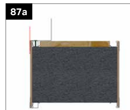
87a Before fitting roof gable panels, pre fit supplied steel angle bracket/s WPCA/2, aligning with the outer edge of the half clip (these could be in 2 lengths dependant on panel length). Align the upper bracket with the top edge of the gable panel and the second bracket (if required) against the first. Secure using the GPHS050 screw.
