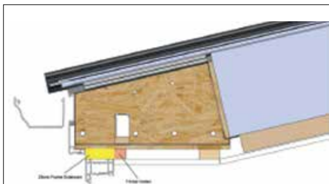
This image is the plaster line detail when at 12.5° using 25mm frame extensions.
