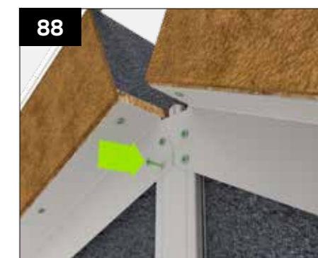
88 Fit gable panels to the top of the wall panels, pushing the steel bracket against the external clips. Secure to the wall panel clips using the provided GPHS050 screws through the pre punched holes.
