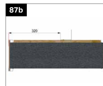
87b If an extended soffit has been specified, measure from the external edge of the panel by 320mm and mark a line. Align the steel angle bracket/s with this line and secure into the OSB using the GPHS050 screw.
