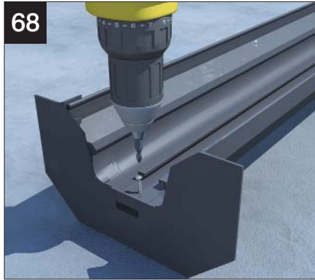
68 Screw the flashing trim to the ridge top cap through the screw port. Use a 4.2mm x 13mm self drilling screw (not supplied).
