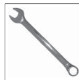
17mm Open Ended Spanner - Tie Bars
