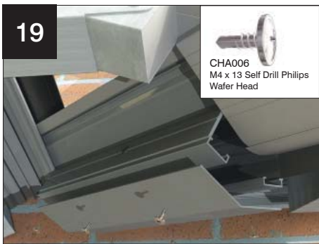
19 Fit valley plate at top of valley using fixings at max 250mm centres.
