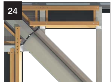
24 Fit adjacent panels by the same method as previous step. Again, terminating the battens at the centreline of the steel undercladding to allow the fixing of adjacent battens in the following steps. (Detail at wall plate shown)
