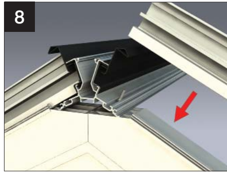
8 Place the starter bars onto the beam top caps and secure to the ridge and eaves beam. Securely fix the starter bars to the beam - screw through at an angle as illustrated to ensure a solid fixing into the aluminium reinforcement.
