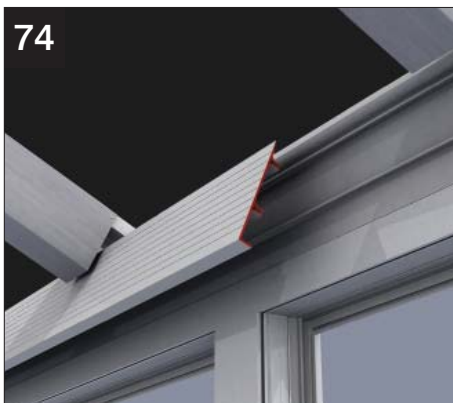
74 Attach fascia board to barbs built into the eaves beam.
