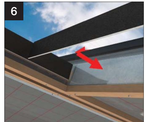
6 Fit black multiboard - ensure it touches glass. Screw fit.
