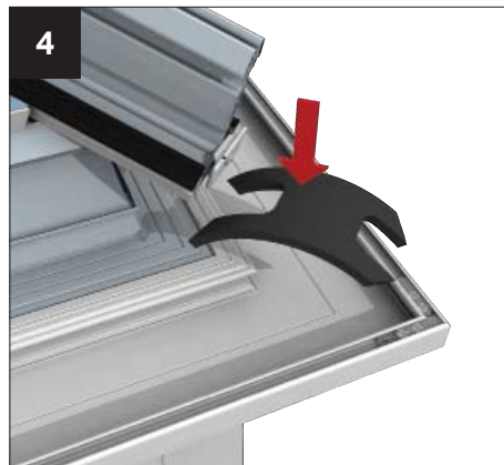
4 At 90° corner insert 'H' section and press down. Similarly apply at stop end or outlet positions.
