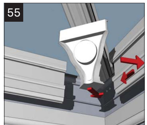
55 Fit the corner covers by trapping them behind the fascia sections. Insert the circular infill to finish.
